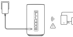
Indicators will turn on when 5G CPE has successfully connected to a network.
